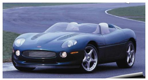
TWO OF THESE 2-SEAT ROADSTER CONCEPT CARS WERE BUILT BY JAGUAR IN 1998/99. DESIGNED BY KEITH HELFET, THEY WERE POWERED BY A SUPERCHARGED JAGUAR QUAD-CAM V8, 450 H.P., 5-SPEED AUTOMATIC GEARBOX. THE ORIGINALS ARE UNOBTAINABLE, BUT REPLICAS ARE BEING BUILT BY MYRTLE LTD. IN BRITAIN. PRICE?? PHONE AND FIND OUT FOR YOURSELF (SEE
