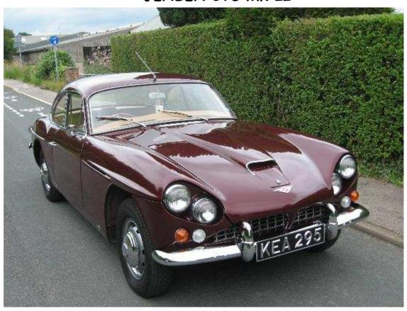
IN ANY REVIEW OF UNUSUALLY-STYLED BRIT CARS, THE JENSEN CV8 MUST BE ONE OF THE FIRST EXAMINED. PRODUCED FROM 1961-66, USING CHRYSLER'S 5.9 OR 6.3 LITRE V8, IT COUND RUN 0-60MPH IN 8 SECS AND TOP 130 MPH. NOW, ABOUT THAT "CHINESE EYE" STYLING......
