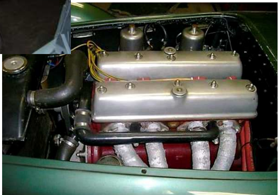
THE RILEY 2.4 LITRE ENGINE AS USED IN THE SILVERSTONE
